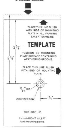
a. Fasten closer to mounting plate using only the screw hole nearest the pivot shaft. The two remaining mounting screw holes will not be used.
