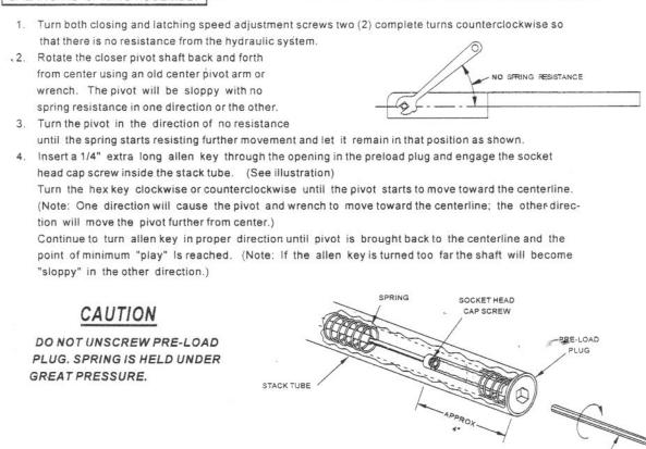
Install closer assembly and hand door. Re-adjust closing and latching speeds for proper door operation. (See page 3)
